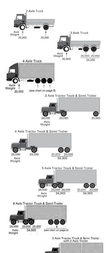
Maximum gross weight is determined by the number of axles and the distance between the first and last axles.
