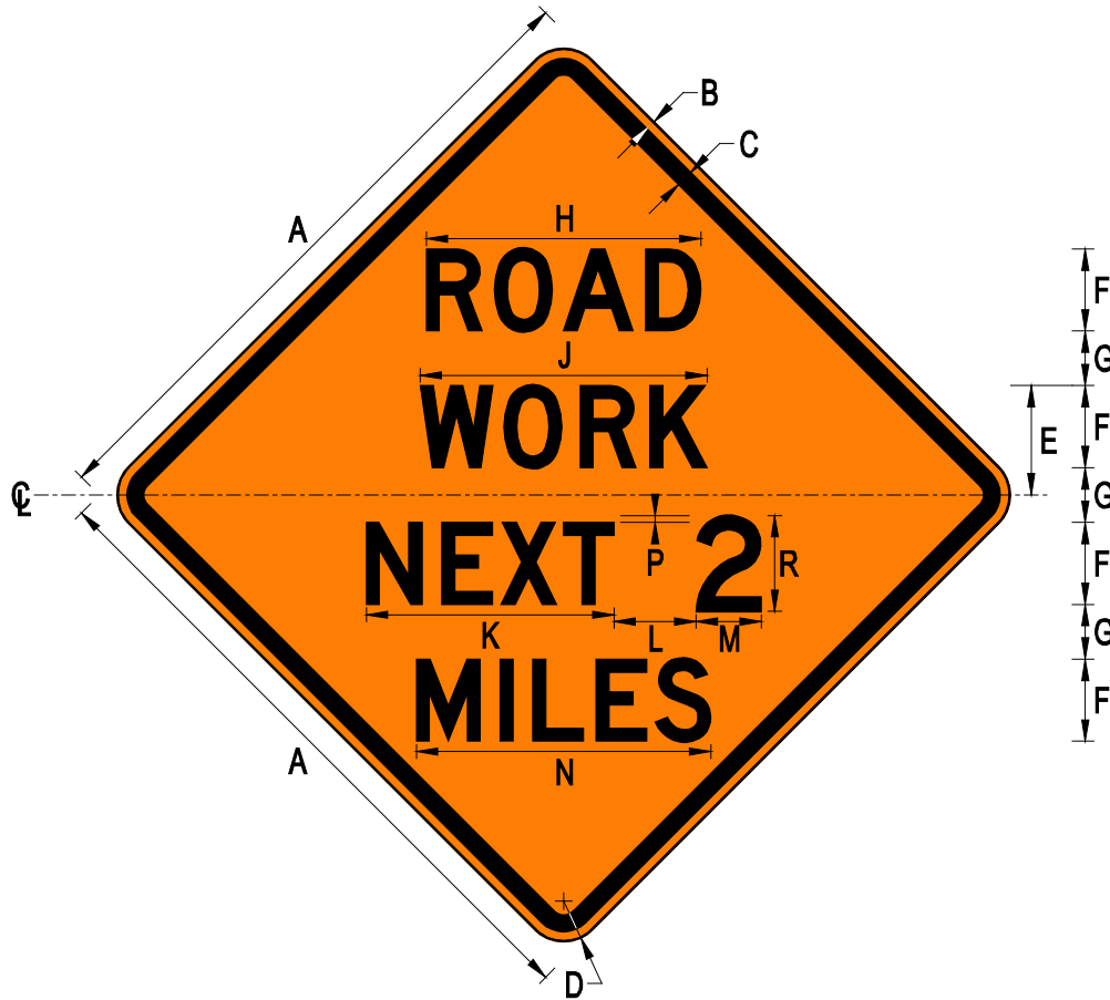
W21-V2 ROAD WORK NEXT 2 MILES
