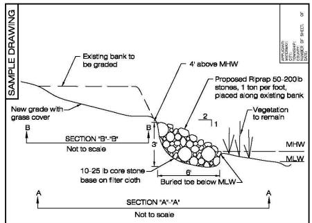
Riprap Revetment & Associated Backfill
