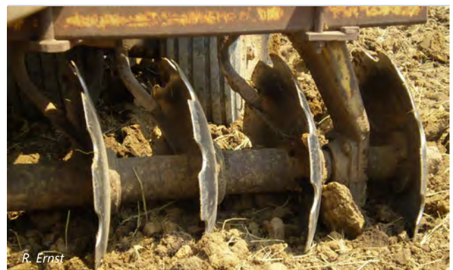
Figure 4-2: Example of disk plowing methods.
